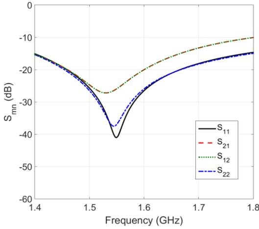
Fig. 4. Reflection and coupling of the two-port *Antenna II*.
