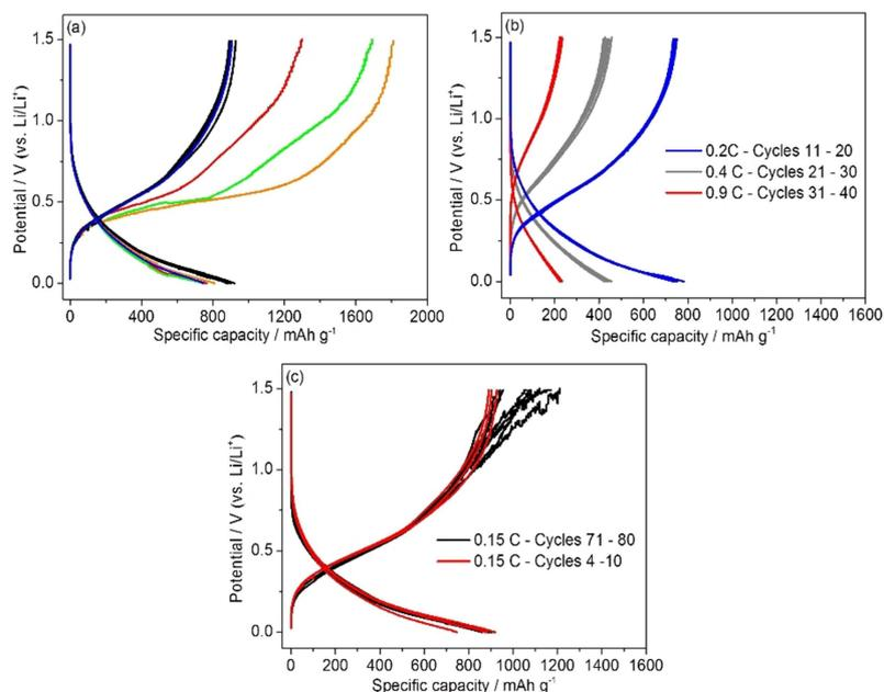
**Figure 6.** Galvanostatic cycling data obtained for 100 nm Ge with  $320\text{ }\mu\text{m}$  thick PG-60, (a) initial charge/discharge cycles obtained at 0.15 C, where the red data corresponds to cycle 1, green to cycle 2, orange to cycle 3, black for cycles 4 to 9 and blue for cycle 10, (b) subsequent cycles obtained at 0.2 C (blue), 0.4 C (grey) and 0.9 C (red), (c) comparison of initial (red) and final (black) charge/discharge cycles obtained at 0.15 C.
