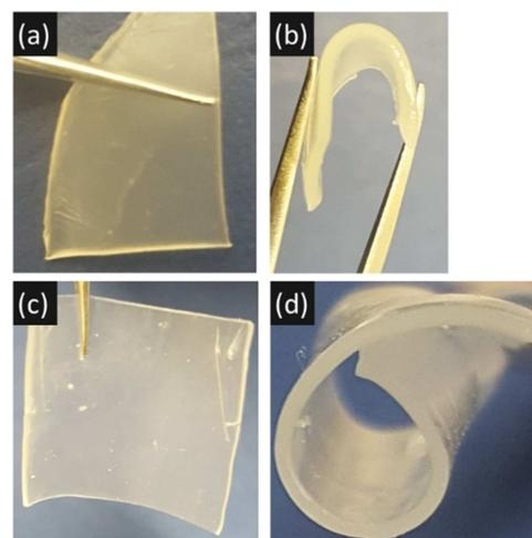
**Figure 1.** Optical images of synthesised 400  $\mu\text{m}$  thick polymer gel electrolytes (a and b) PG-10, and (c and d) PG-60. Films of various thicknesses were synthesised and 42  $\mu\text{m}$  films were used and discussed below for Figure 5.
