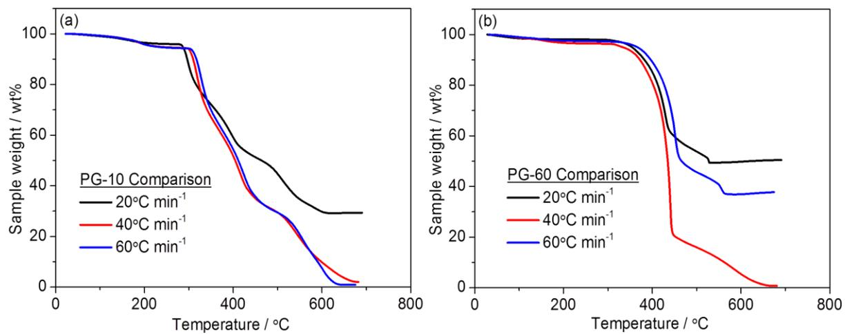
**Figure A4.** TGA data where PG-10 and PG-60 were analysed under air. The temperature was ramped by 20°C min<sup>-1</sup>, 40°C min<sup>-1</sup> and 60°C min<sup>-1</sup>. The thermal stability for each of the gels remains similar for each temperature ramp which demonstrates that the polymer gels are stable under different temperature conditions.
