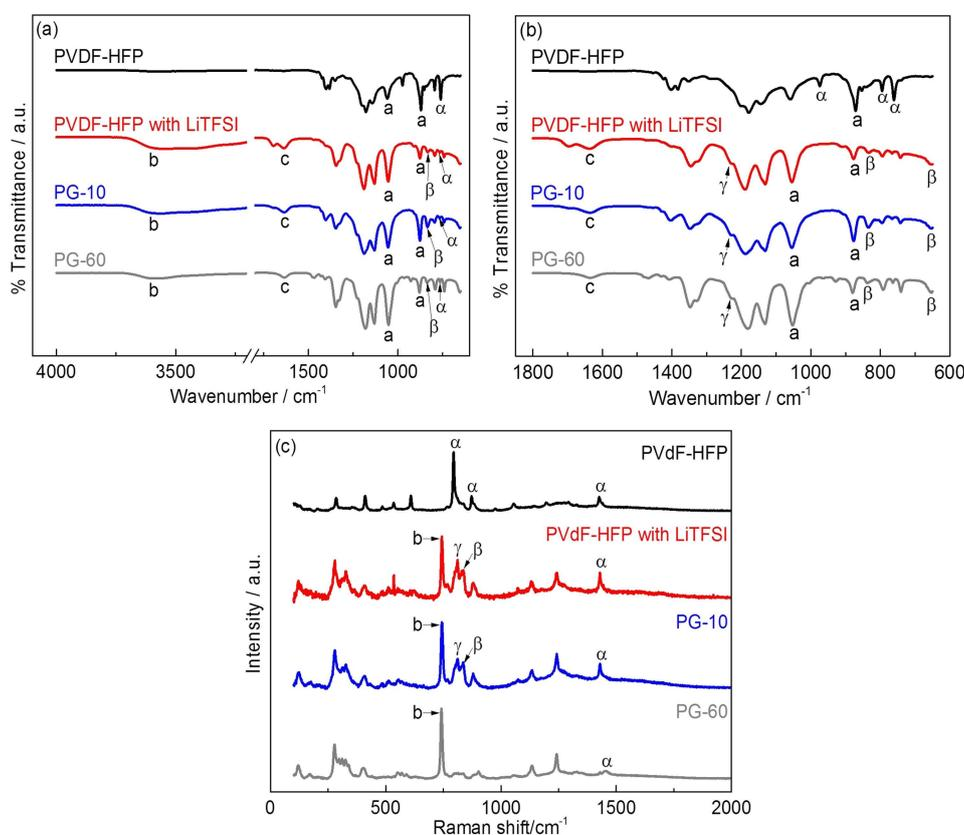
**Figure 3.** Room temperature FT-IR spectra of PVDF-HFP, PVDF-HFP with LiTFSI, PG-10 and PG-60, (a) displaying the range 4000  $\text{cm}^{-1}$  to 650  $\text{cm}^{-1}$ , (b) displaying the range 1800  $\text{cm}^{-1}$  to 650  $\text{cm}^{-1}$ , (c) room temperature Raman spectra of PVDF-HFP, PVDF-HFP with LiTFSI, PG-10 and PG-60.
