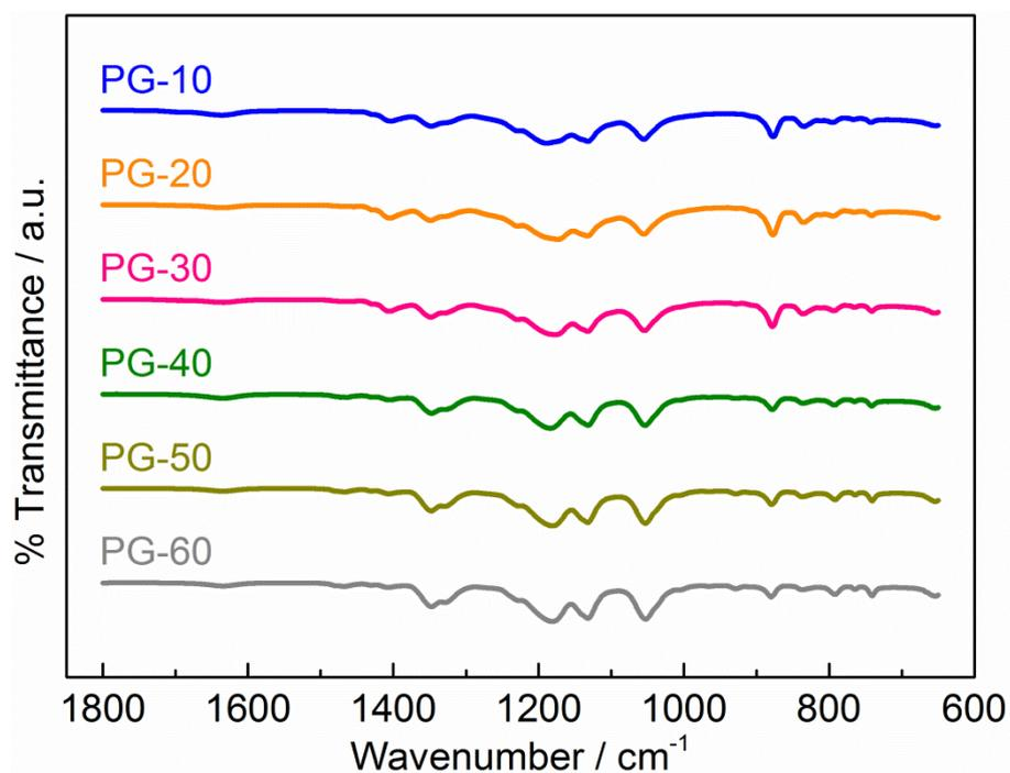
**Figure A2.** FT-IR data for the polymer gel series where the  $C_4\text{mpyrTFSI}$  content was increased from 10% to 60%. Similar crystalline states were observed for the series of polymer gels, where amorphous,  $\alpha$ -phase,  $\beta$ -phase and  $\gamma$ -phase were all observed. Peak assignments are given in section 3.3.
