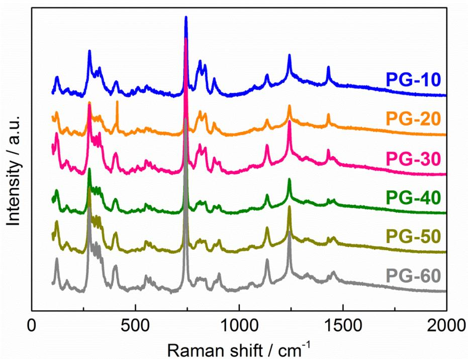
**Figure A3.** Raman data for the polymer gel series where the  $C_4\text{mpyrTFSI}$  content was increased from 10% to 60%. As the  $C_4\text{mpyrTFSI}$  content was increased, the intensity of the  $\beta$ - ( $836\text{ cm}^{-1}$ ) and  $\gamma$ -phase ( $811\text{ cm}^{-1}$ ) peaks decrease as the film becomes amorphous. The intensity of the peak at  $743\text{ cm}^{-1}$  increases as the  $C_4\text{mpyrTFSI}$  content increases due to the higher TFSI concentration in the polymer gel.
