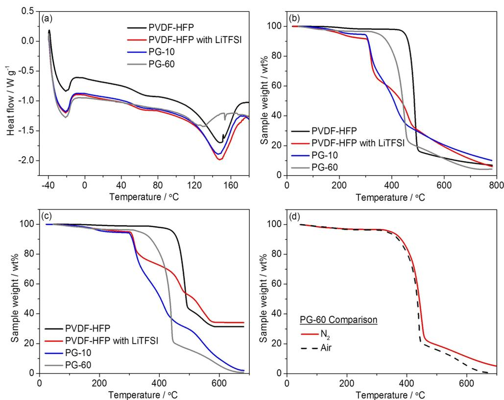
**Figure 4.** (a) DSC traces of pure PVDF-HFP, PVDF-HFP with LiTFSI, PG-10, and PG-60, (b–d) TGA plots obtained under (b)  $\text{N}_2$  and (c) air, where the  $\text{N}_2$  flow rate was  $10 \text{ ml min}^{-1}$ , (d) comparison of TGA plots for PG-60 obtained under  $\text{N}_2$  and air.
