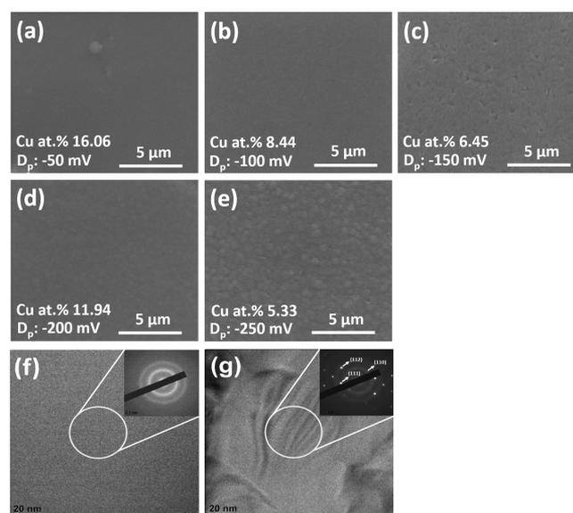
**Figure 3.** SEM and TEM micrographs of Cu-doped Te films at (a)  $-50$ , (b)  $-100$ , (c)  $-150$ , (d)  $-200$ , and (e)  $-250$  mV. (f) TEM image of the film deposited at  $-50$  mV with the SAED inset and (g) TEM image of the film deposited at  $-50$  mV, showing nanofeatures along with the SAED inset.
