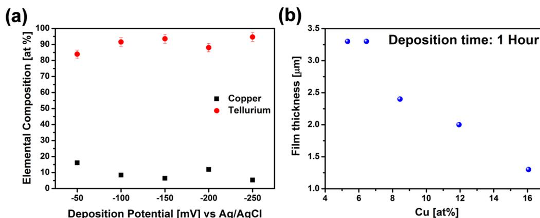
**Figure 2.** (a) Elemental composition of films at different deposition potentials and (b) thickness of electrodeposited films with different Cu atomic percentages.
