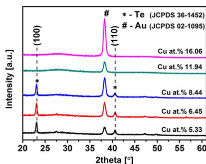
**Figure 4.** X-ray diffraction patterns of the deposited films with increasing Cu at.% in the films.
