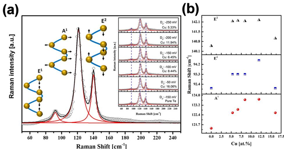
**Figure 5.** (a) Room temperature Raman scattering spectra of films without and with increasing Cu at.% in the films and (b) Raman spectra peak shift of A<sup>1</sup>, E<sup>1</sup>, and E<sup>2</sup> peaks.
