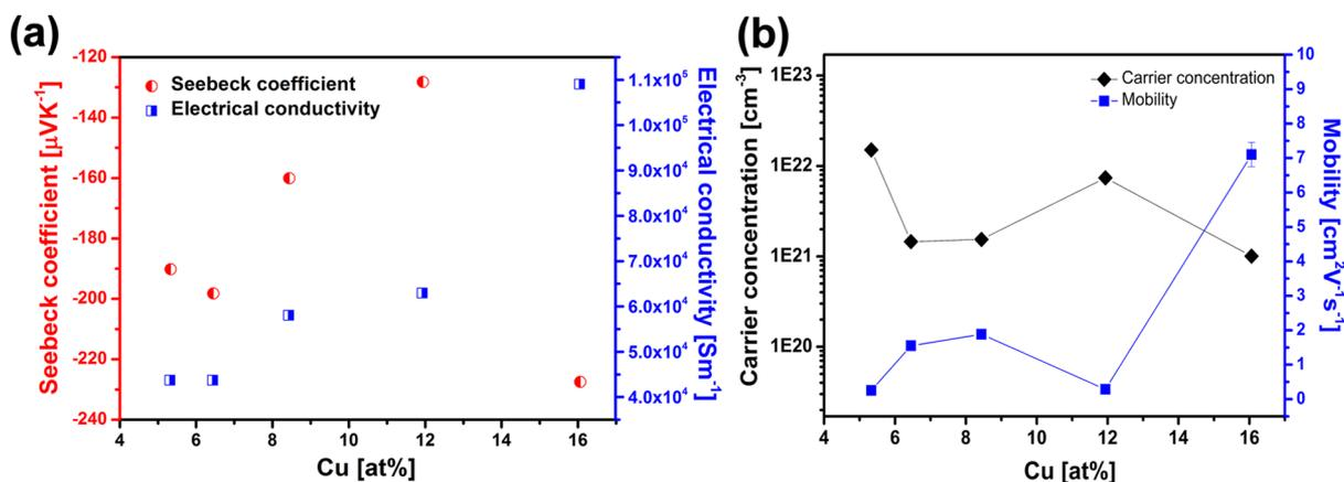
**Figure 6.** (a) Thermoelectric properties of electrodeposited Cu-doped Te films with different Cu contents in the films, and (b) mobility and carrier concentration as a function of Cu atomic percentage in the films.
