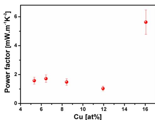
**Figure 7.** Calculated power factor of the films with different Cu at.% in the films.
