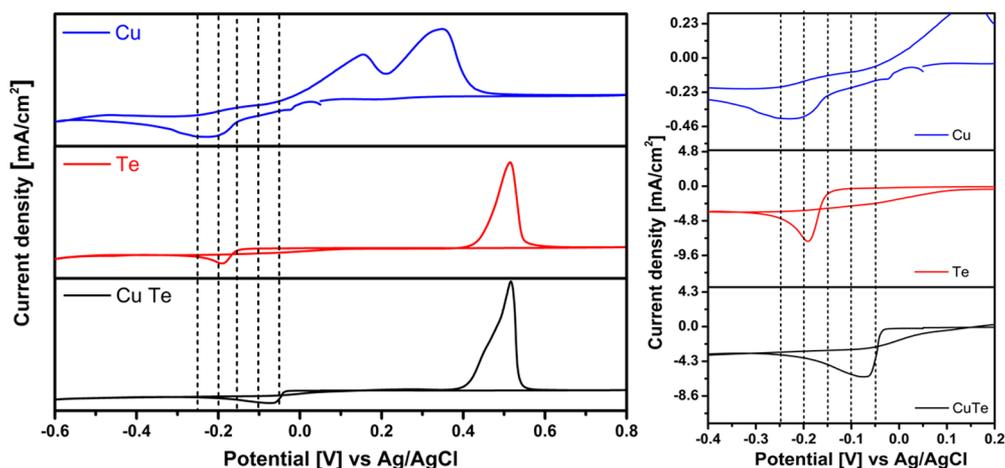
**Figure 1.** Cyclic voltammogram recorded on a standard gold working electrode in the Cu, Te, and CuTe electrolytes, and a magnified image of reduction peaks (right).
